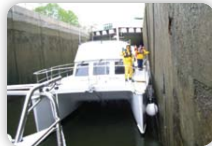
Wide decks allow for ease in handling lines in locks and for docking
