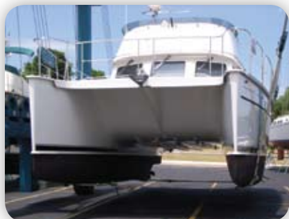
Wide stance of the catamaran hull means stability
